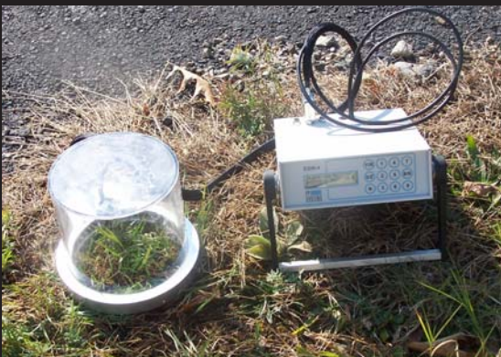
The CPY-4 shown above with the EGM-4 Environmental Gas Monitor for CO 2
